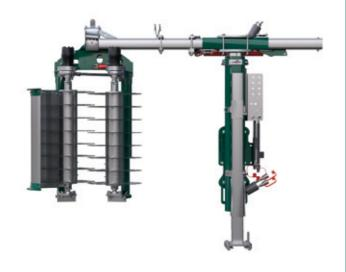
The pre-pruner is used to remove the one-year-old wood and can be used in cordon systems as well as for spur pruning. The cutting head is equipped with a different number of cutting pairs depending on the conditions. The distance between the knives is 100 mm. This dimension can be reduced to half or increased by using different spacers.
