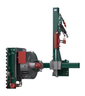
The leaf remover is used for mechanical defoliation of the grape zone and can be used from flowering until shortly before harvest. The leaves are sucked in by a suction roller and plucked off by a roller rotating in the opposite direction. The leaves are blown forward into the row by a fan.
