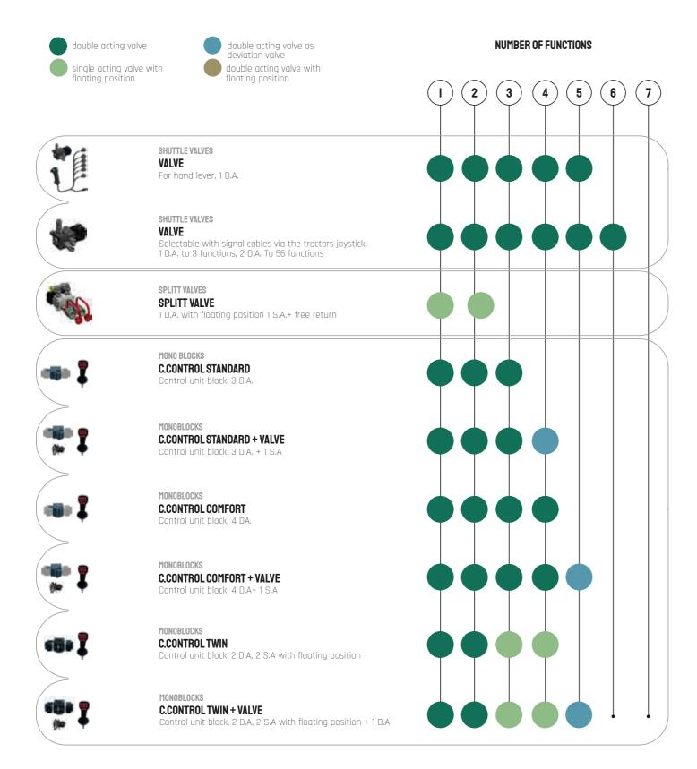
You do not have enough control valves on your tractor to operate different hydraulically driven implements or adjustment functions at the same time? With the C.DRIVE system, we offer you a convenient and cost-effective solution.
