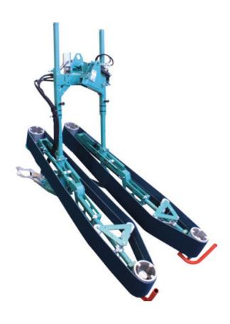
The shoot binder EASYFIX is easy to use, maintain and adjust and works with biodegradable clips. This means that after about 18 months of exposure to the sun, the polypropylene stapling cord can be mechanically removed with a rewinder, saving a significant amount of time.
