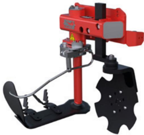
RADIUS SL AROUND-THE-VINE WEEDER is the environmentally friendly alternative to chemical weed control. The weeds rot in a natural manner. Less drought stress through destruction of the roots. Soil activation and promotion of optimum soil condition. Sensitive sensor technology for clean work around the vine. Rear, mid and front mounting possible, 1 or 2 sided versions. Versatility through different tools in front of the blade and additional devices.
