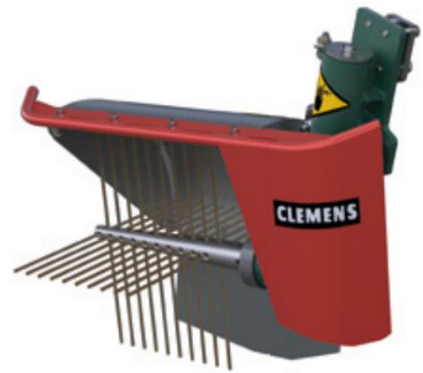
The mulching brush has very strong and smooth cords that protect the vine. The conical aluminum shaft operates smoothly and with little vibration because of its special shape. It is therefore possible to carry out weeding effectively at 1100 rpm. With the MULTICLEAN you can remove both the water shoots and the weeds simultaneously with one machine.
