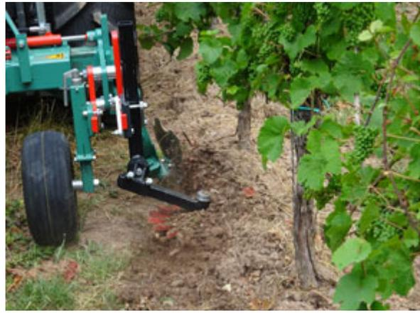
As advantages of this equipment are speed and, if you use it skilfully, trouble-free combination with other steps of work. Used frequently, small banks could be built unintentionally. To reduce this effect, we would suggest using the combination of both **finger roller / GSP-disc** and **finger hoe**. Another possibility is to work with the share and the **finger roller** together.
