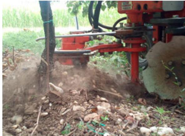
By this combination, the soil will be broken up by the share, than crumbled by the rotating tiller. Depending on the rotational speed of the tiller, the ground will be also cleared up from the row.
