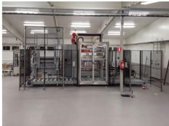
A new product line is being built, that will later de-palletize the empty bottles, then fill and label them and at last palletize and stretch-wrap the finished cartons fully automatically.
