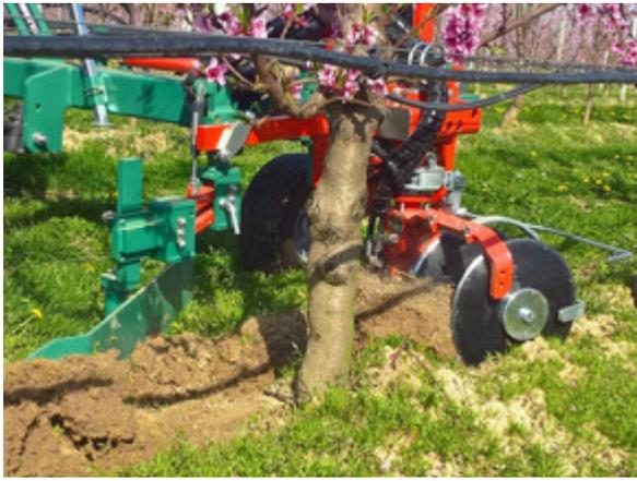
The rotating discs (2 pieces diameter 410 mm) are used to pull out the soil from the space between the two rows, to level up, to make furrows, to fertilize and to manure. The rotating discs are equipped with a metal plate to protect the vine from possible damages, in case the sensor rod should not work properly.
