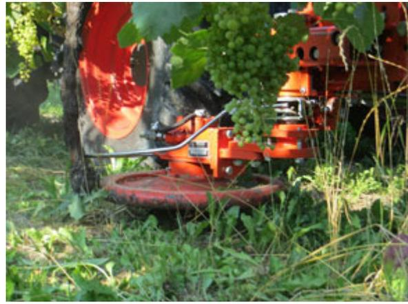
The mower (400) waves by a hydraulic motor between the vines. A rubber ring protects the plants.
